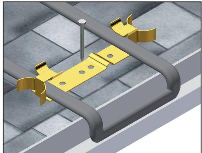
1. Plan the layout of the roof clips according to the installation instructions supplied with the cable. One double clip is used to secure the hearing cable looped at the roof edge ( this assures a drainage channel to the gutter). A single clip is used to fasten the cable at the tip of the saw tooth layout arrangement Single clips are made by snapping the double clip in two at the scored indentation.
