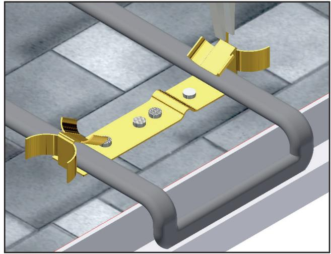
3. After installing the clips on the roof, thread the heating cable around the clips. Used extra clips in any location where the heating cable is susceptible to excess stress or movement.
