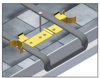
Fasten the clips to the roof with roofing nails or screws. Apply water sealing material around the nail/screw to prevent water leakage.
