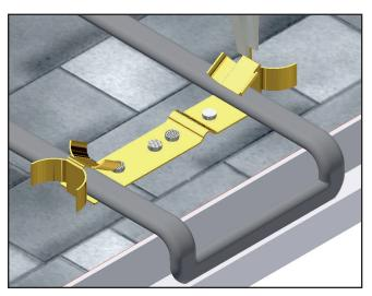
Using pliers, close the clips firmly around the cable, being careful not to crush the cable.
