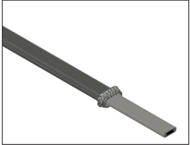
2. Push the braid back to expose the inner jacket on the base cable.
