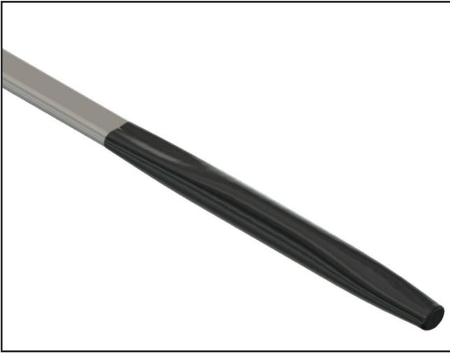
9. Apply heat evenly to the heat shrink tube until it shrinks around the cable. While it is still hot, gently squeeze the end of the shrink tube with pliers and hold until cool. The end must remain visibly sealed when the pliers are removed.
