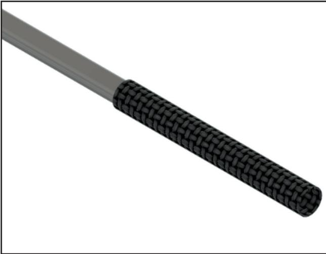
7. Slide the 4" woven braid sleeving over the end of the cable, allowing at least 1/2" to extend past the end of the cable.
