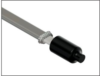
4. Slide the heat shrink cap over the end of the cable.
