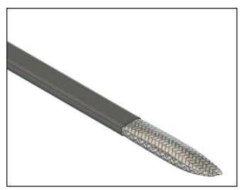
6. Pull the pushed back braid over the sealed end cap and twist the braid together at the end.
