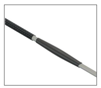
**10.** Push the braid splice against the insulated cable splice. Center the 5" heat shrink tube (Item 2) over the braid splice/cable splice. Apply heat evenly until the tube shrinks down around the connection. Allow to cool.
