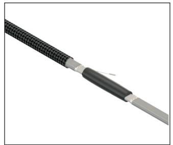
**8.** Apply heat evenly until the tube shrinks down around the cables and connectors. The adhesive should flow from both ends. Allow the tubing and adhesive to cool before going to the next step.
