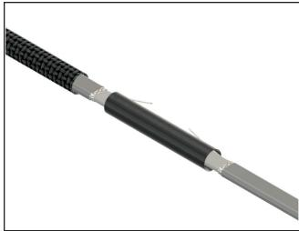
7. Center the 3" long heat shrink tube (Item 4) over the insulated barrel connectors, being careful to keep the pigtails out from under the shrink tube.
