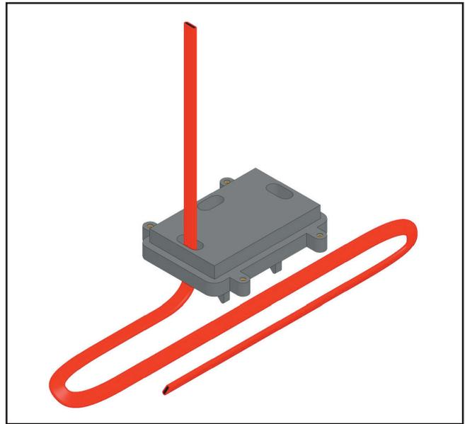
3. Secure the base to the pipe by threading the appropriate sized pipe strap through the slot in the mounting plate. Tighten the pipe strap until the base is securely attached to the pipe.
