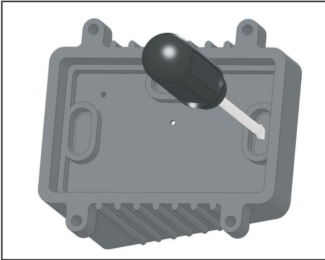
2. Feed the ends of the cables through the appropriate hole in the base. Allow 8" of cable to extend above the top of the base.
