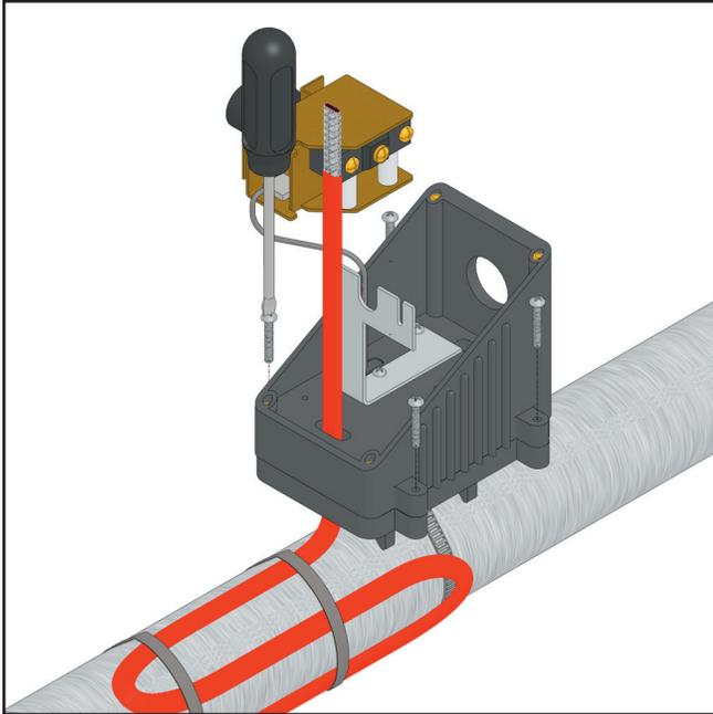
6. Starting from the end of the cable, unravel 1-1/2" of the braid. Twist the strands together to form a pigtail.
