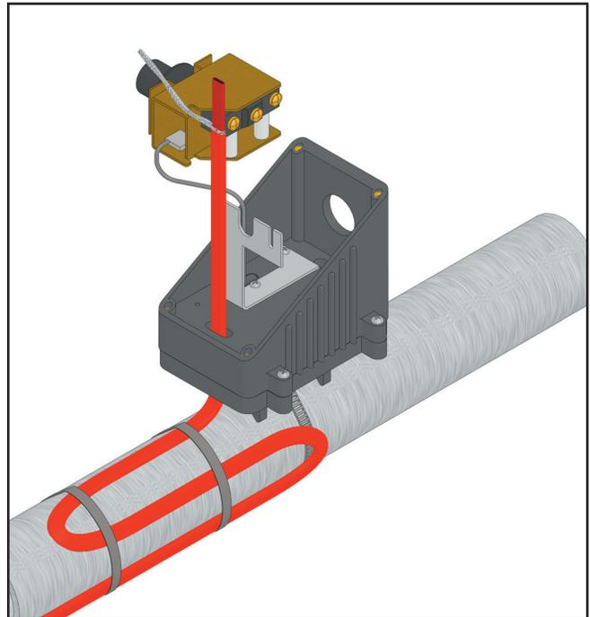
7. Using standard electrical cutters, cut a 3/4" long notch out of the cable between the conductor wires. Bare a 3/8" length of each conductor by stripping off the outside insulation and the inner black core material.
