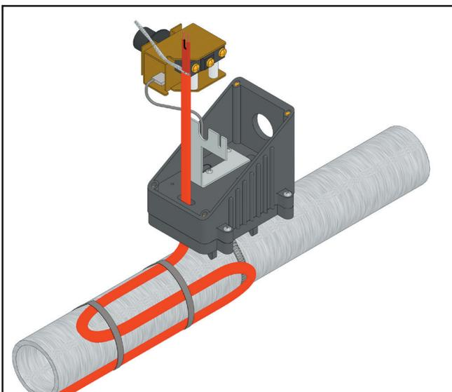
8. Insert the bared ends of the conductors and the braid into the openings in the terminal block. Tighten screws firmly to hold the wires in place. Attach UL certified conduit to hub and bring power leads into box. Strip 3/8" length of each power wiring. Connect conduit hub (Chromalox CCH-1, CH-75 or equal) to the box. Attach conduit to hub and bring 8" of power leads into the box.
