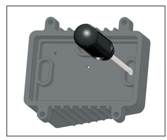
1. Use a hammer and screwdriver to punch out the knockouts on the bottom of the box which correspond to the openings in the base through which the heating cable passes. Only punch out the knockouts that are to be used. If one is mistakenly punched, blank grommets can be ordered to reestablish the water tight seal.
