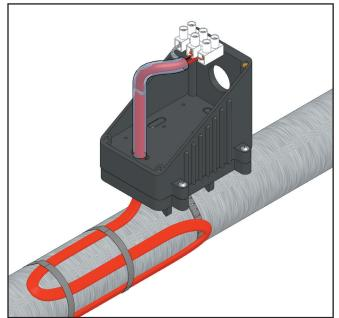
8. Slide the 6" insulation tubing over the cable. Insert the bared ends of the conductors and the braid into the openings in the terminal block. Tighten screws firmly to hold the wires in place. Connect conduit hub (Chromalox CCH, CH-75 or equal) to the box. Attach conduit to hub and bring power leads into box. Strip 3/8" length of each power wiring. Crimp the ring connector onto the end of the "Hot" conductor.
