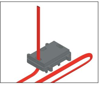
**2.** Feed the ends of the cables through the appropriate hole in the base. Allow 8" of cable to extend above the top of the base.
