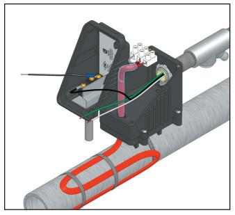
9. Make sure water tight rubber gasket (Item 6) is in place. Remove the screw and collar from the NOR-MALLY CLOSED terminal of the thermostat. Discard the collar. Push the screw through the opening in the connector attached to the insulated wire and screw it back into the terminal. Remove the screw and collar from the COMMON terminal. Discard the collar and push the screw through the opening in the ring connector. Drive the screw back into the COMMON terminal.
