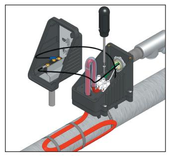
**11.** Mount terminal block to bottom of the box by driving the self-tapping screw (Item 11) provided into the mounting hole as shown.
