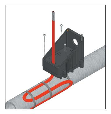
5. Feed cables through the corresponding holes in the box and secure box to base using all four of the 1" long screws.
