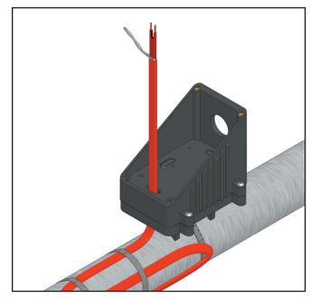
7. Using standard electrical cutters, cut a 3/4" long notch out of the cable between the conductor wires. Bare a 3/8" length of each conductor by stripping off the outside insulation and the inner black core material.
