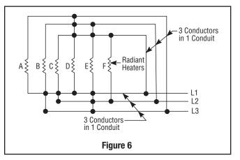
Three phase Delta connections to minimize inductive effect in conduits are made per this diagram. The rule: run all 3 three-phase conductors in the same conduit as far as possible. For single-phase, run only two conductors and follow the same rule.
