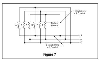
Three phase Delta connections to minimize inductive effect in conduits are made per this diagram. The rule: run all 3 three-phase conductors in the same conduit as far as possible. For single-phase, run only two conductors and follow the same rule.
