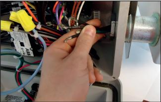
**12.** Connect black jumper wires to contactor terminals and green jumper wire to ground lug.
