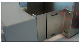
9. Attach Slotted Mounting Bracket (Item C) to Base Mounting Bracket by inserting (2) 5/8 x 10-32 machine screws (Item F) through slots and into threaded holes. Secure using remaining 8-32 k-nuts (Item G). Fully tighten.
