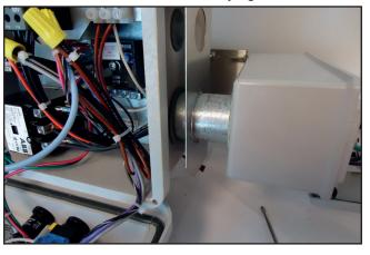
Place lock washers on 1-1/2 x 8-32 machine screws (Item E) and insert into Disconnect Housing Assembly.
