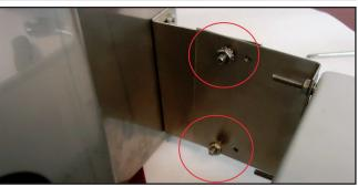
**Note:** There are 4 threaded holes on the Base Mounting Bracket to allow for assembly to be installed on different heater housing sizes. 2-20kW heaters should use threaded holes farthest from the L-bend in the bracket and 25-39kW heater should use holes closest to the L-bend.
