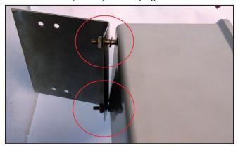
Secure Slotted Mounting Bracket (Item C) to heater frame using (2) 5/8 x 10-32 machine screws (Item F). Fully tighten.
