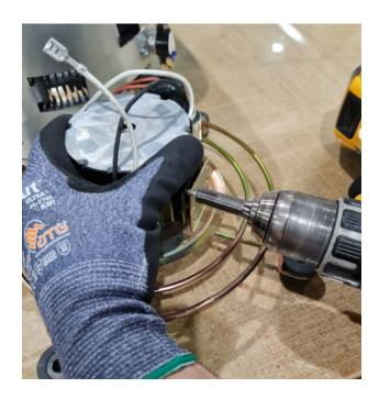
Don't forget to install the ground wire prior screwing in the screw on the Motor's bracket.
