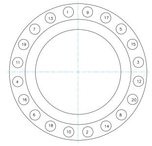
A tightening sequence similar to that shown in Figure 2 is recommended for use until any angular misalignment is taken up. When flange faces are parallel the tightening sequence shown in Figure 1 shall be used.
