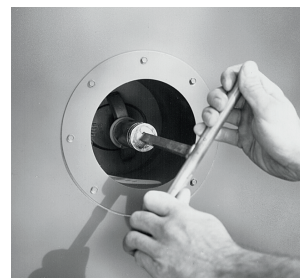
FIGURE 6 - REMOVING HAND ASSEMBLY WITH TEE HANDLE WRENCH
